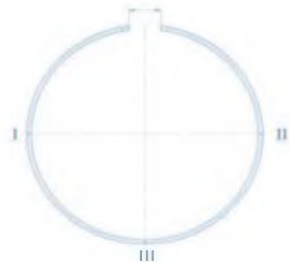
Fig. 1 – Areas for observing changes in piston ring lock size and coercive force
