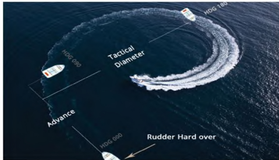
Fig.3 – Advance and tactical diameter during turning of vessel
