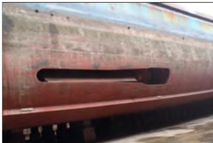
Figure 4 – Portside fin stabilizer recess
