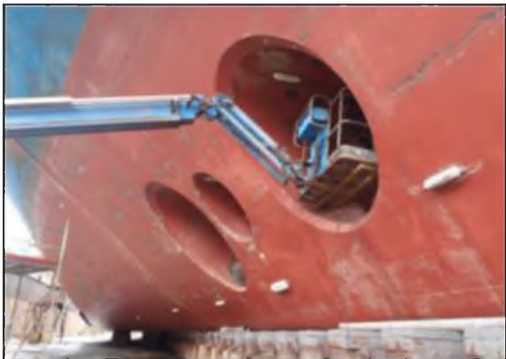
Figure 1 – Bow thrusters (starboard side view) and Anti-suction tunnel (AST)
