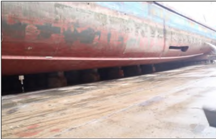
Figure 6 Portside bilge keel
