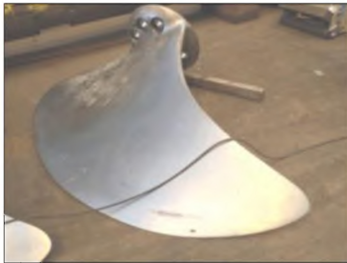
Figure 10 – Propeller blade. A streak of cavitation damage can be observed on the pressure side (near the lower edge in the photo)
