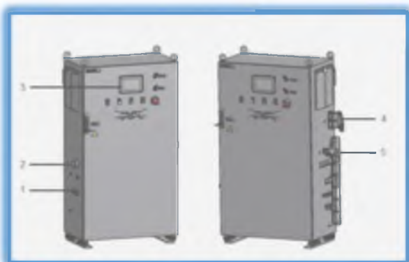
Figure 12 – Electrical cabinet with main control panel:
